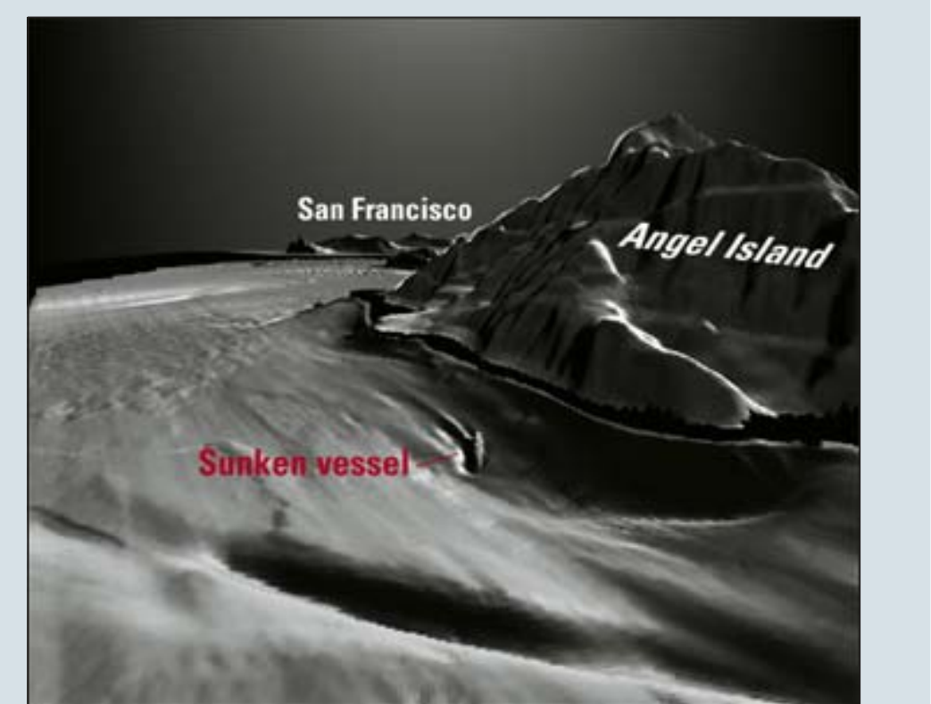
A sunken vessel can be seen in this view of the floor of San Francisco Bay northeast of Angel Island. The presence of this object was already known to the U.S. Coast Guard, but its identity has not been determined. This image was created from the recently collected bathymetric data (for the bay floor) and USGS topographic data (for the land). View is from the north, looking south toward San Francisco.
