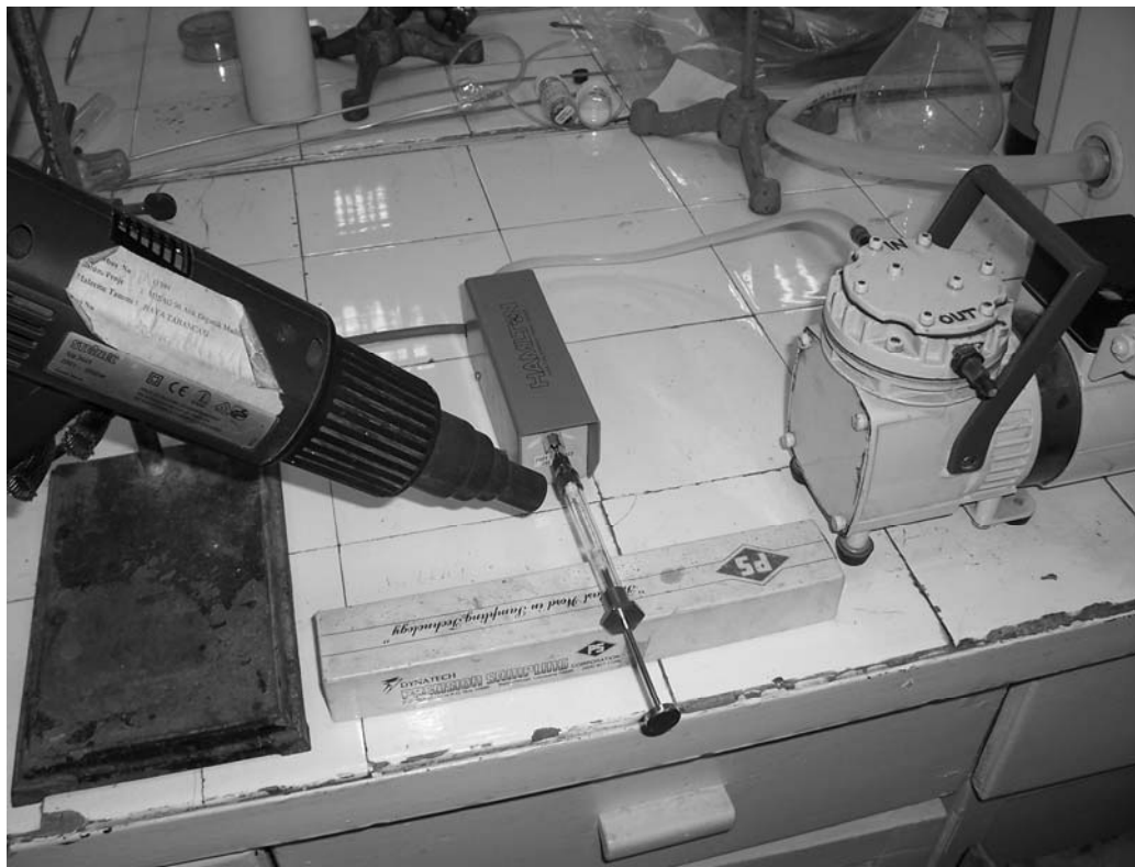
Figure 8. Heating gun (left) and syringe cleaning equipment
