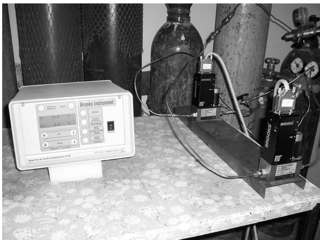
Figure A.14. Gas cylinders and mass flow controllers
